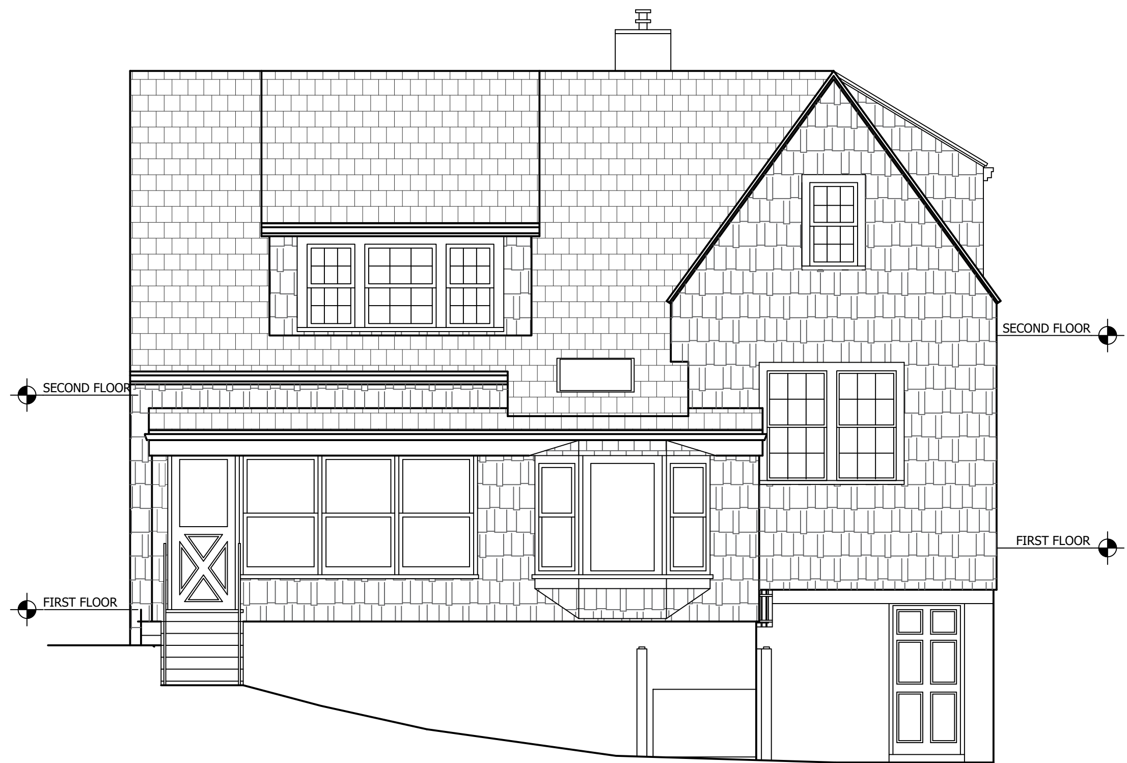
1 EXISTING REAR ELEVATION SCALE : 1 / 4" = 1'-0"
