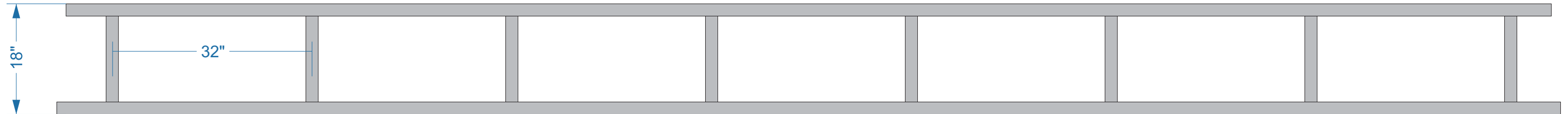
3 Sign Frame (1) 2" Aluminum Tube Frame w/ Sunbrella Fabric 3/4" = 1'-0"
