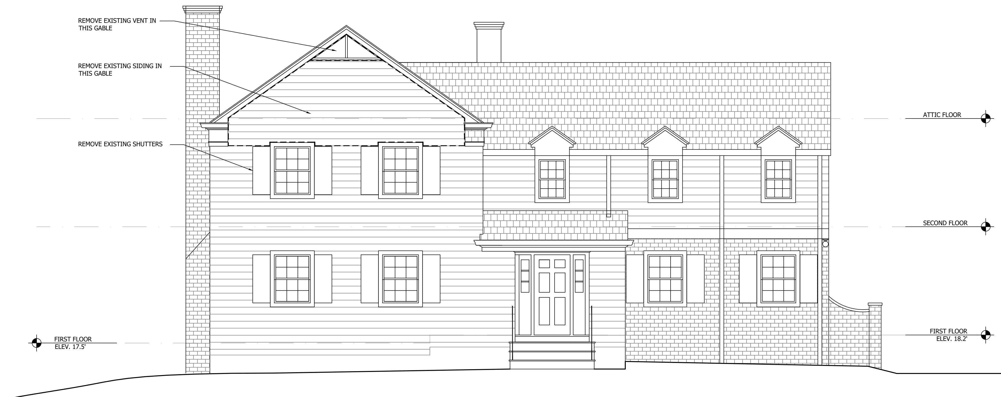
1 EXISTING FRONT ELEVATION SCALE : 1 / 8" = 1'-0"
